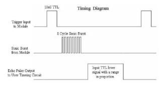
Distance Equations for sensors  $D = (\Delta t/2) x c$
