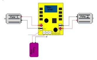
One of the most well-known DC motor drivers is the L298N dual H-bridge motor driver. This driver allows the circuit designer to control the speed as well as the direction of the DC motor. The L298N driver also consists of heat sinks for high current loads. It also incorporates motor direction LED indicator. Most of the DC motors lie within the operating voltage range of 5 to 35VDC. Therefore, this driver is ideal for all such motors.
